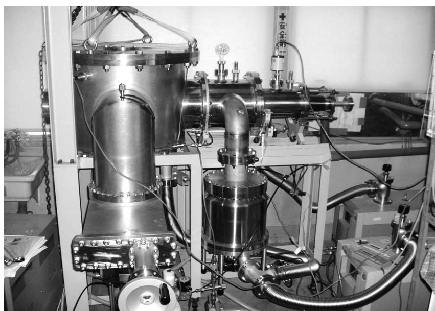
図4-1 Vacuum chamber developed to make a molecular beam
